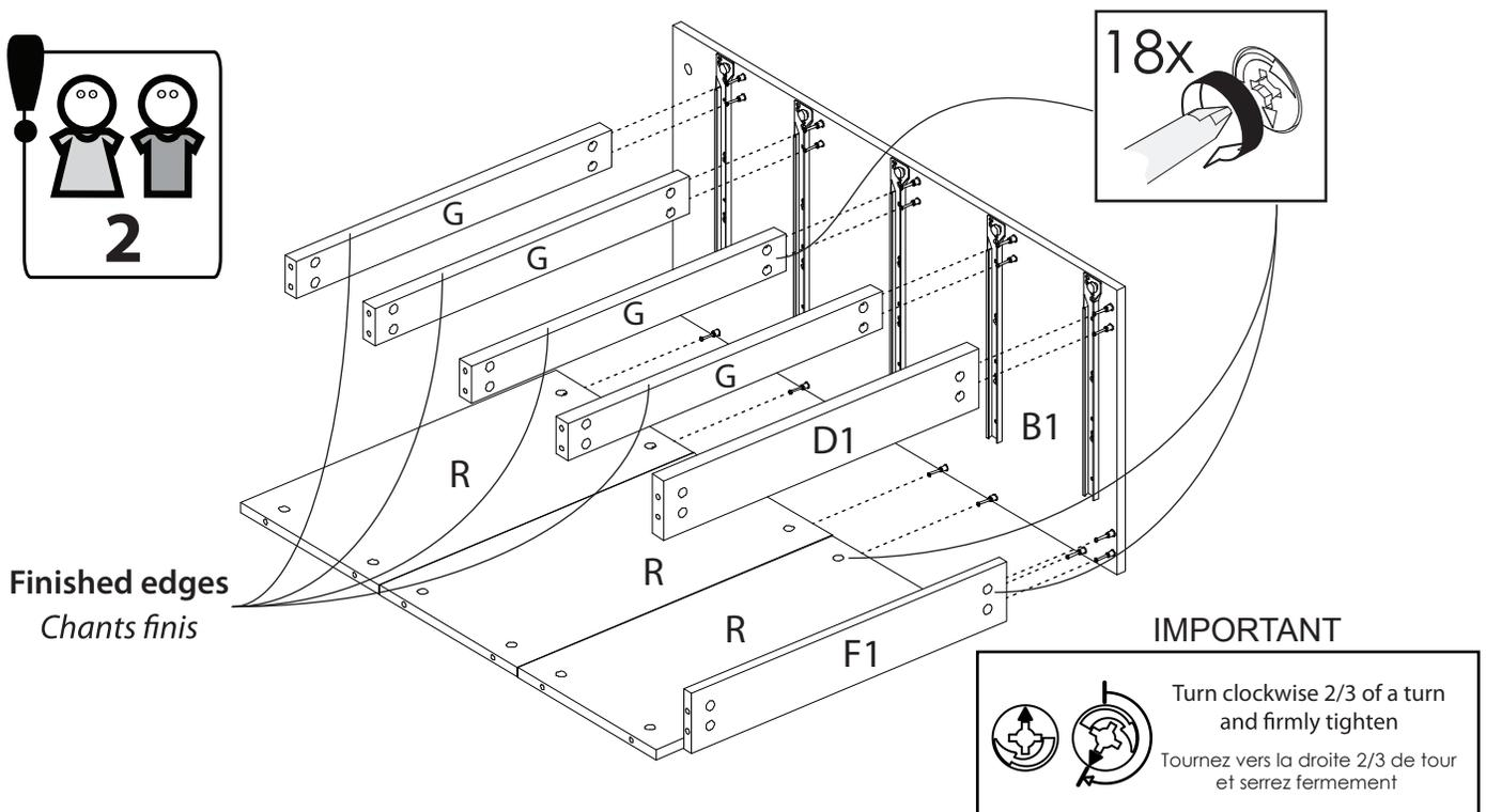
**5** Fasten the panel A1 to the assembled unit. Then, tighten the 18 cam locks # 0203 located on the panels D1, F1, G and R
