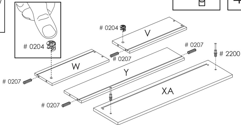
**8** Fasten the panels V and W to the drawer front XA and tighten the 2 cam locks # 0204
