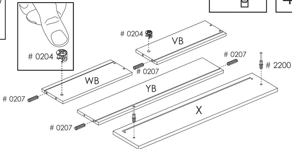
**13** Fasten the panels VB and WB to the drawer front X and tighten the 2 cam locks # 0204
