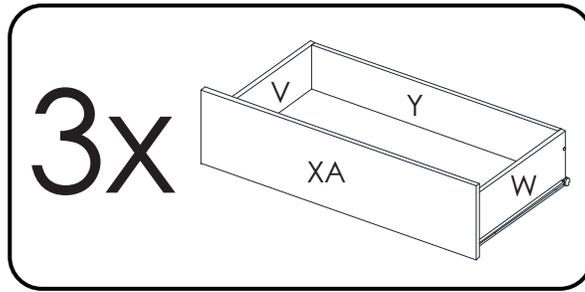
**7** Install 2 small cam locks # 0204 on panels V and W. Install 2 push bolts # 2200 on panel XA. Install 4 wood dowels # 0207 on panels V, W and Y
