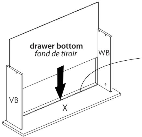
**Drawer bottom must enter into the groove located on panel X**
