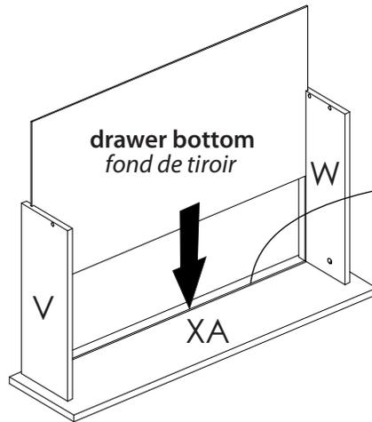
Drawer bottom must enter into the groove located on panel XA
