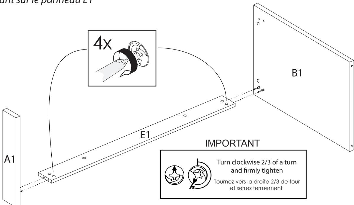
**4** Fasten the panel C1 to the assembled unit. Then, tighten the 6 cam locks # 0203 located on panels A1, B1 and E1
