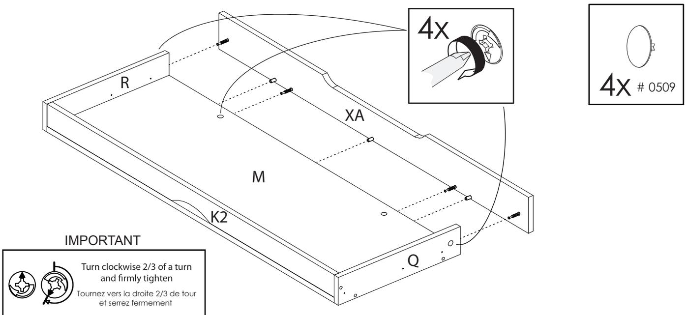
**11** Use the 6 screws # 0105 to fasten the 2 drawer slides # 0917 to the panels Q and R
