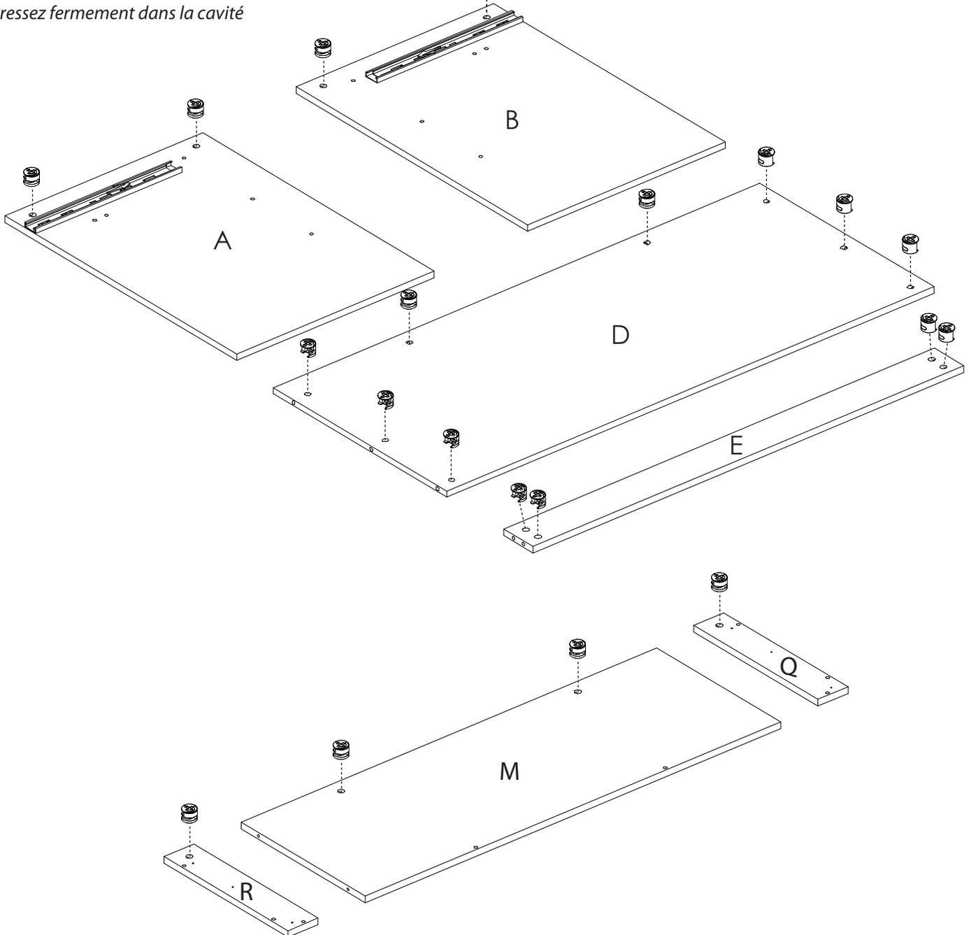
**3** Install the 16 push bolts # 2200 on panels A, B and C
