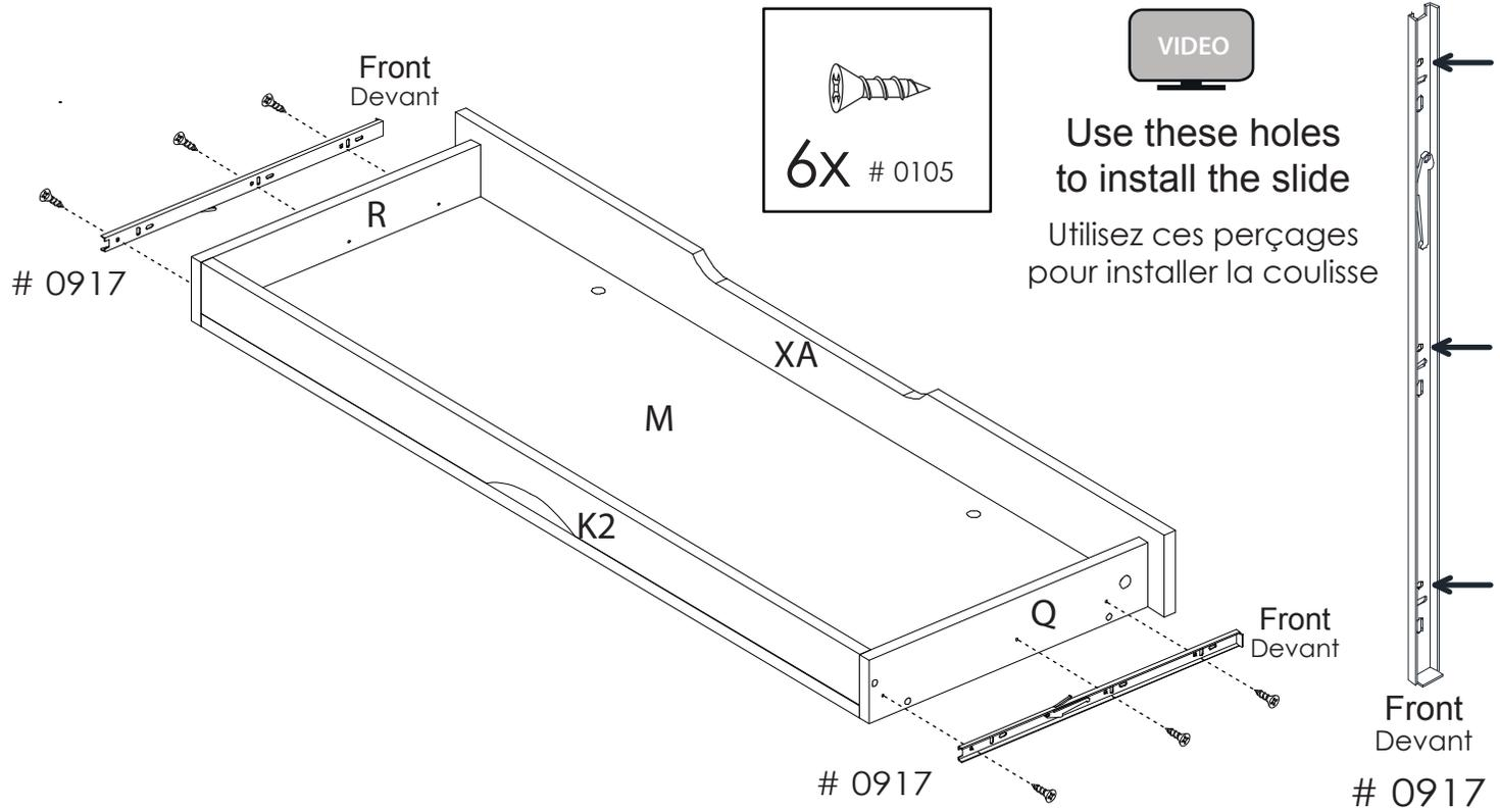
**12** Insert carefully the drawer into the assembled unit
