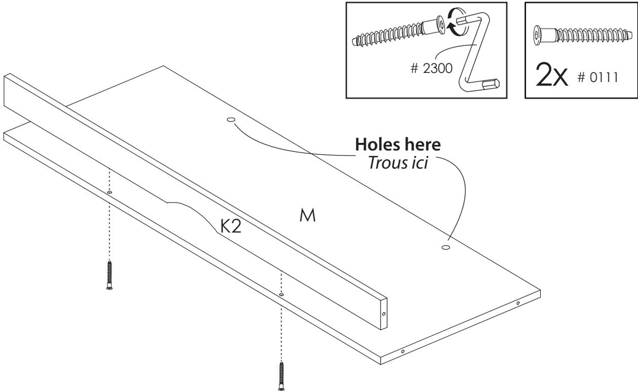
**8** Use the Allen key # 2300 and 6 screws # 0111 to fasten the panels Q and R to the assembled panels K2-M
