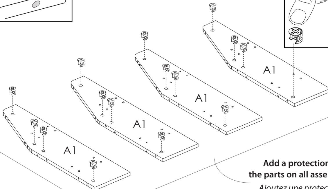
**Add a protection under the parts on all assembly steps**
