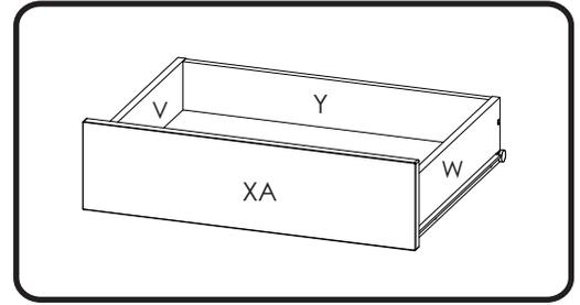
**10** Install 2 small cam locks # 0204 into panels V and W. Install 2 push bolts # 2200 into the panel X or XA. Insert 4 wood dowels # 0207 into panels V, W and Y
