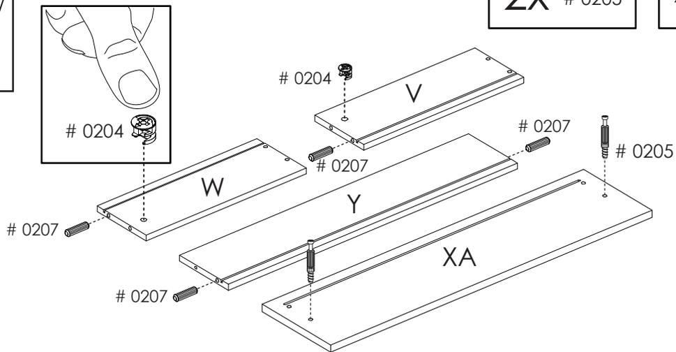
**15** Fasten panels V and W to the drawer front XA and firmly tighten the 2 cam locks # 0204
