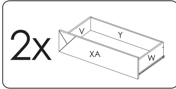
**14** Install 2 small cam locks # 0204 on panels V and W. Install 2 screw bolts # 0205 on panel XA. Install 4 wood dowels # 0207 on panels V, W and Y
