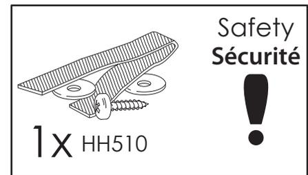
**Attach to the wall with proper anchor device (not included)**
