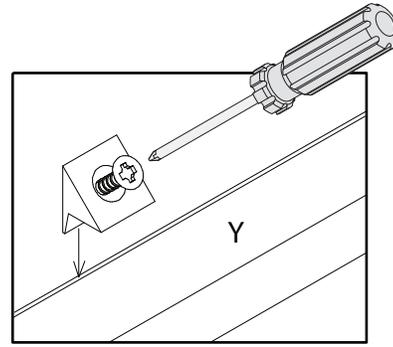
**Insert the small lip of the connector into the groove. Then, hold firmly the connector and screw in place.**
