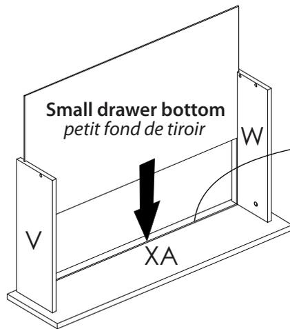
Drawer bottom must enter into the groove located on panel XA
