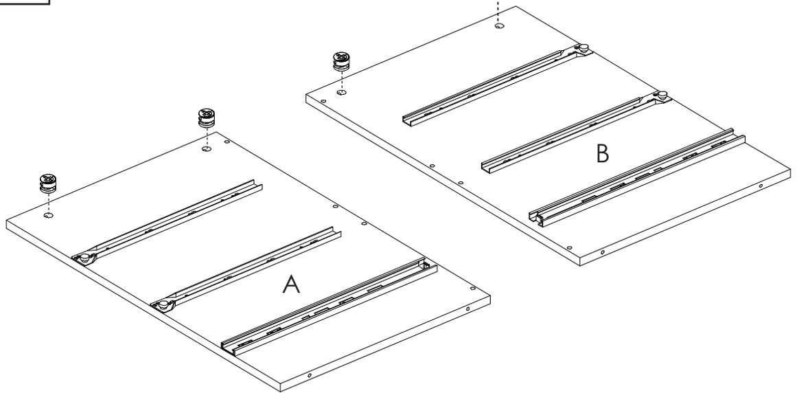
**3** Install 8 wood dowels # 0207 into both panels T
