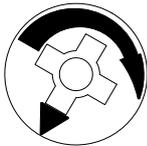
Turn clockwise 2/3 of a turn and firmly tighten
