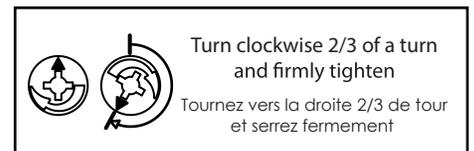
**6** Fasten the panel E to the assembled unit. Then, tighten the 2 cam locks # 0203 located on the panel E. Finalize the step by using the Allen key # 2300 and 2 screws # 0111 to fasten the panel E to the panels G and H
